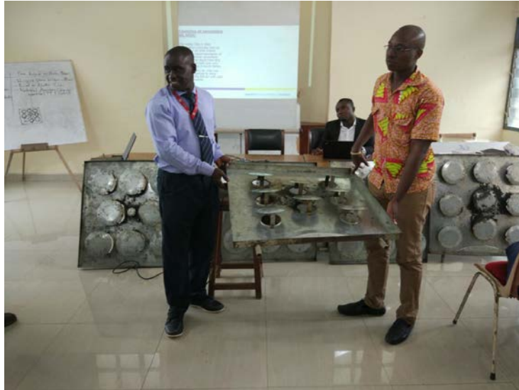
Figure 10: Showing committee members the various types of fat collectors designed for the test
