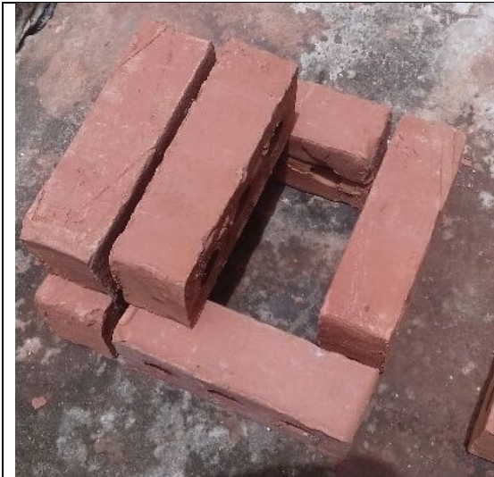
Figure 2: Four bricks on the edge of the combustion chamber to improve heat distribution
