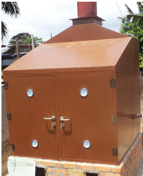
Figure 5: Gas Cabinet Dryer
