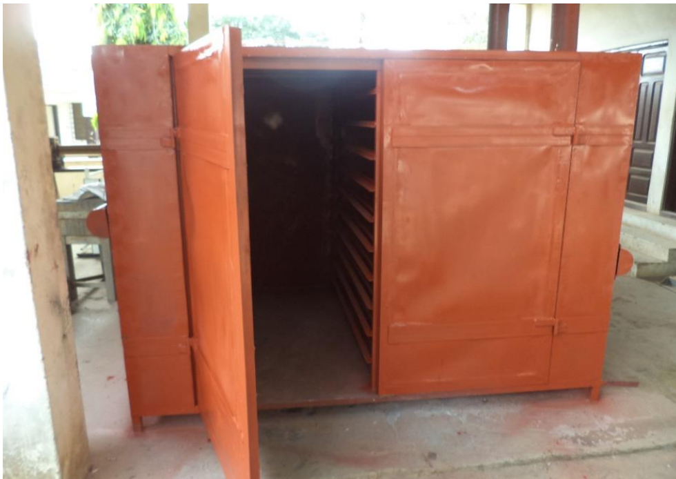
Figure 22: Front view of dryer with doors installed
