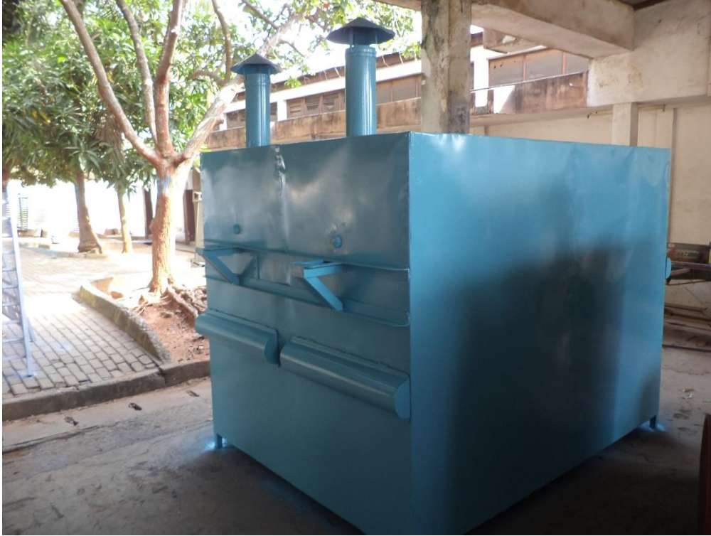
Figure 32: Sprayed painted dryer allowed to dry for about 3 day
