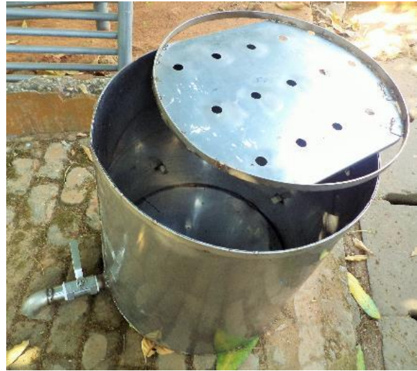
Figure 14. Solid vessel with waste water exit
