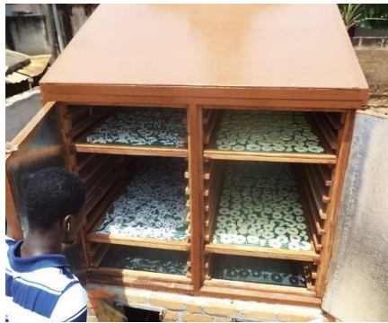
8. Wooden-gas cabinet dryer for fruit drying
