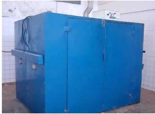
8. Wooden-gas cabinet dryer for fruit drying
