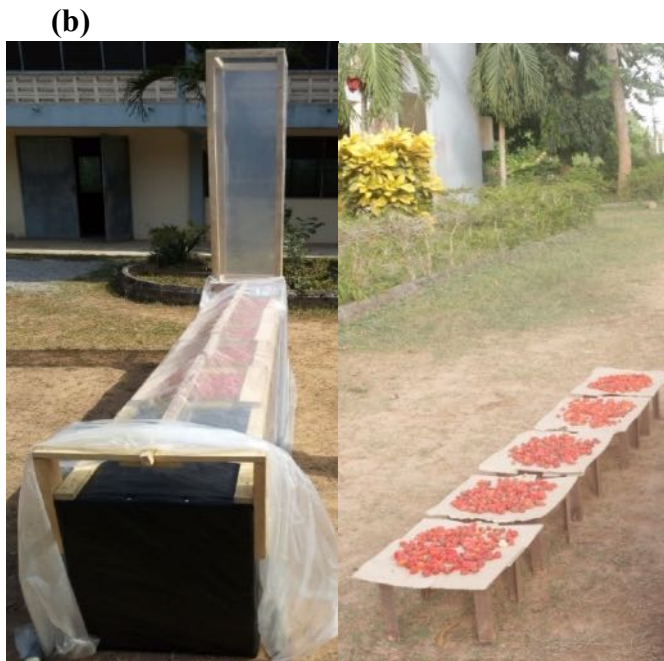
Figure 1: (a) 3-Dimensional drawing of the solar dryer (b) Set-up of the constructed solar dryer with pepper samples in the dryer(left) and the open sun(right)
