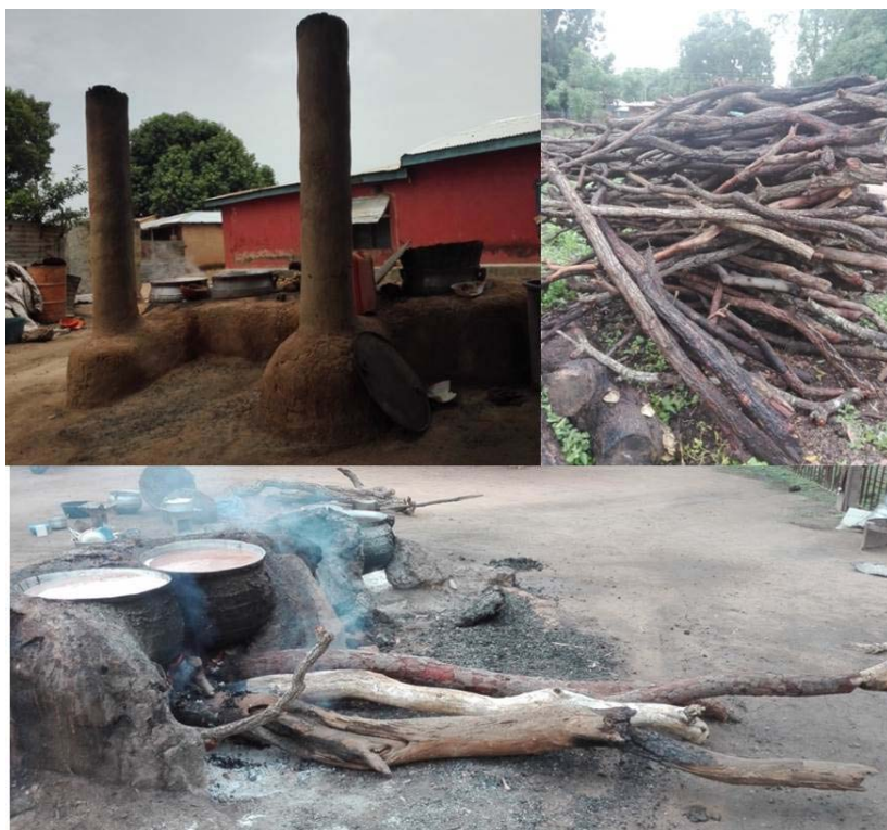
Figure 6-6: Upper left: pito brewing site (oven type), upper right: firewood necessary for brewing 400 L of pito in an open-fire brewing site, below: open-fire brewing site.
