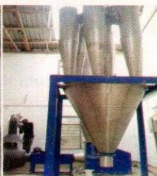
Fully operational flash dryer
