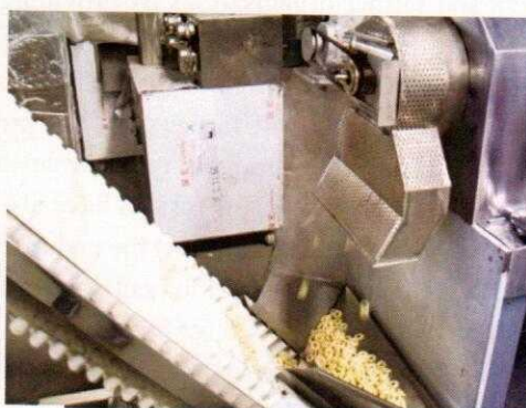
Trial operation of extruder
