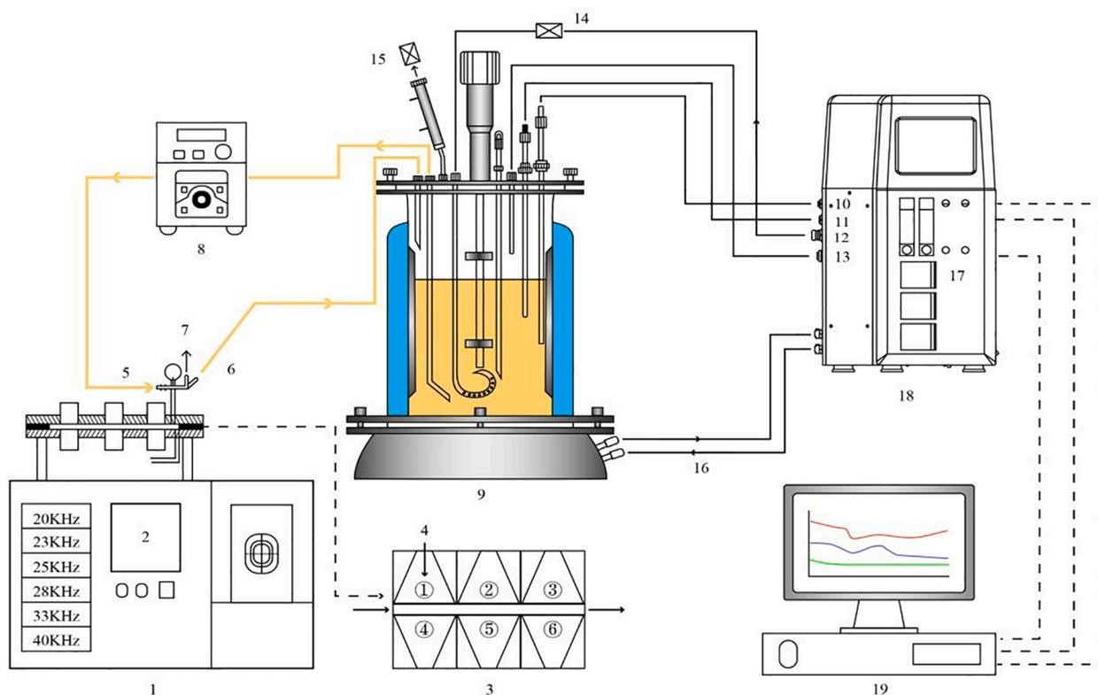
**Fig. 1.** External ultrasound irradiation of broth in a recycle bioreactor (1. Slit ultrasonic equipment 2. control panel 3. Ultrasonic generator 4. Ultrasonic transducer 5. Material liquid inlet 6. Material liquid outlet 7. Sterilization vent 8. Peristaltic pump 9. Fermentation tank 10. Do electrode 11. pH electrode 12. Air flow 13. Temperature Sensor 14. Air filter 15. Exhaust outlet 16. Circulating condensate 17. Electric pump 18. Fermentation tank main console 19. Computer host).
