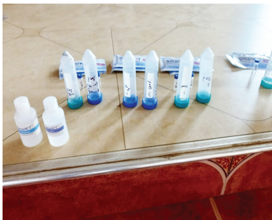
Lateral flow devices, centrifuge tubes and solvent buffers for rapid extraction of aflatoxins
