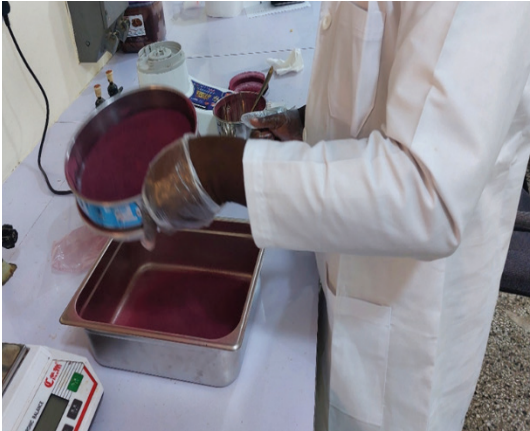
Sieving the milled beetroot powder through a 60-mesh sieve (250 \mu\text{m} )
