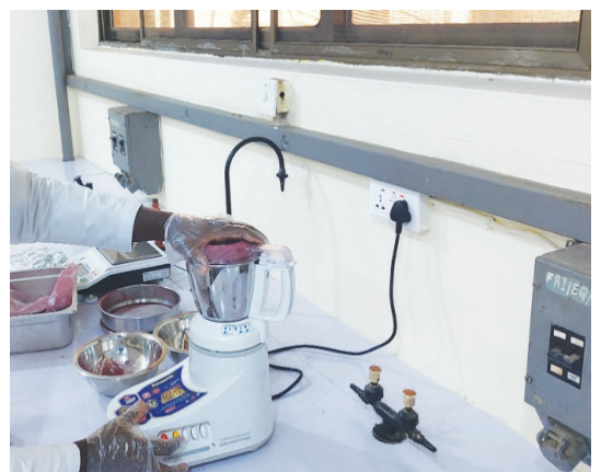
Milling of the dried beetroots into powder using a super mixer grinder
