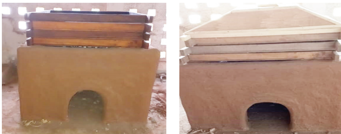
Modified Chorkor oven with fat collector.
