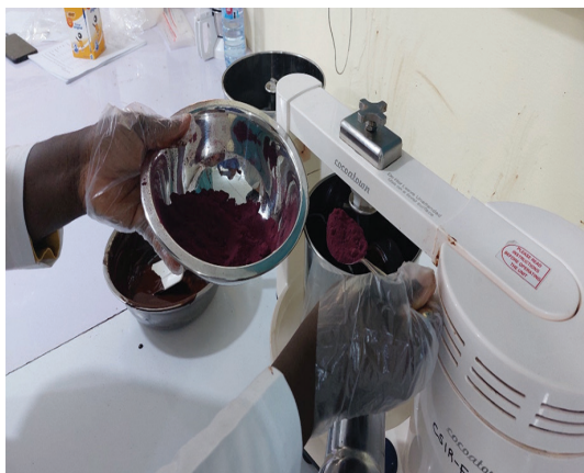
Adding beetroot powder to the cocoa liquor in the melanger during chocolate production
