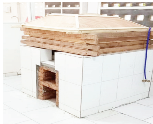
Gas, charcoal and fuelwood combined Ahotor oven.
