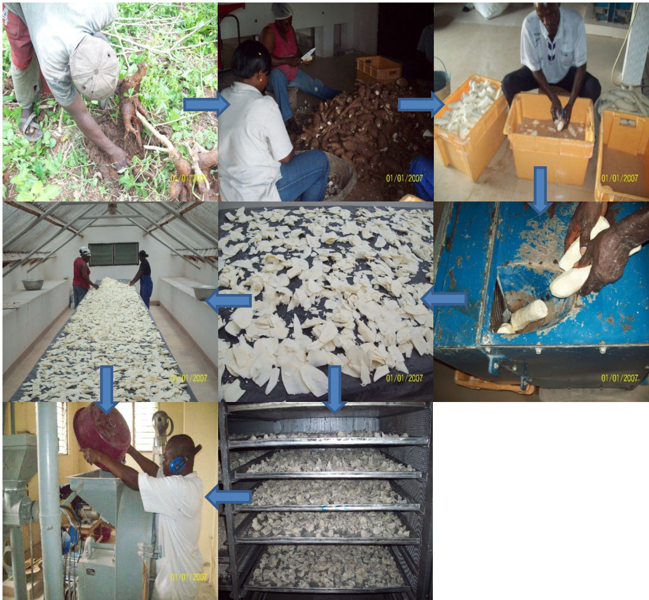
Figure 1b: Processing HQCF by chipping and mechanical/solar drying
