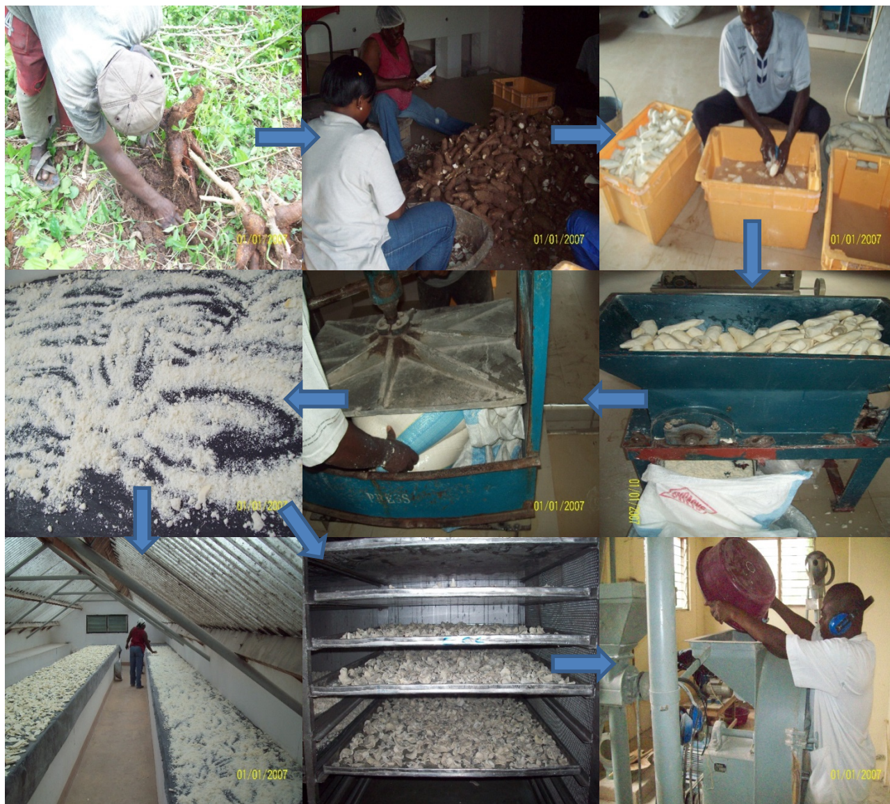
Figure 1a: Processing HQCF by grating and mechanical/solar drying
