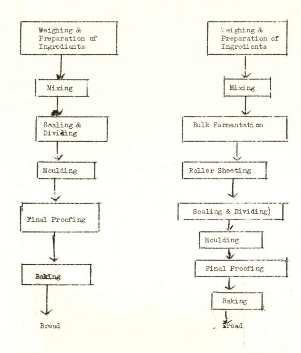
Fig.1 Breadmaking by the Straight-dough method
