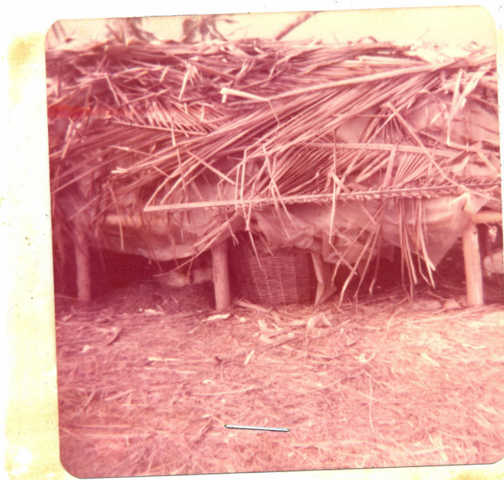
Fig. 13. Covered oven with palm fronds during smoking
