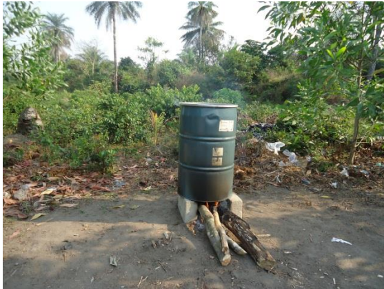
Figure 13: Sterilization being done in oil drums fuelled with firewood
