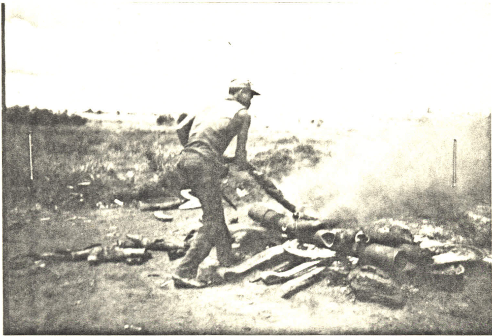
FIG: V. Picture showing evolution of thick black smoke from burning scrap tyres during the singeing of cattle hides.
