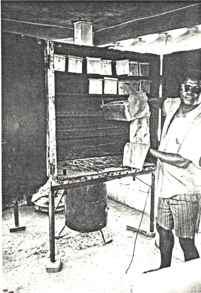
PLATE 10: A saw-dust fired metal oven. Note the rectangular baking chamber, with shelves and chimney; the cylindrical firing chamber; and the heat conducting rods at the base of the baking chamber.
