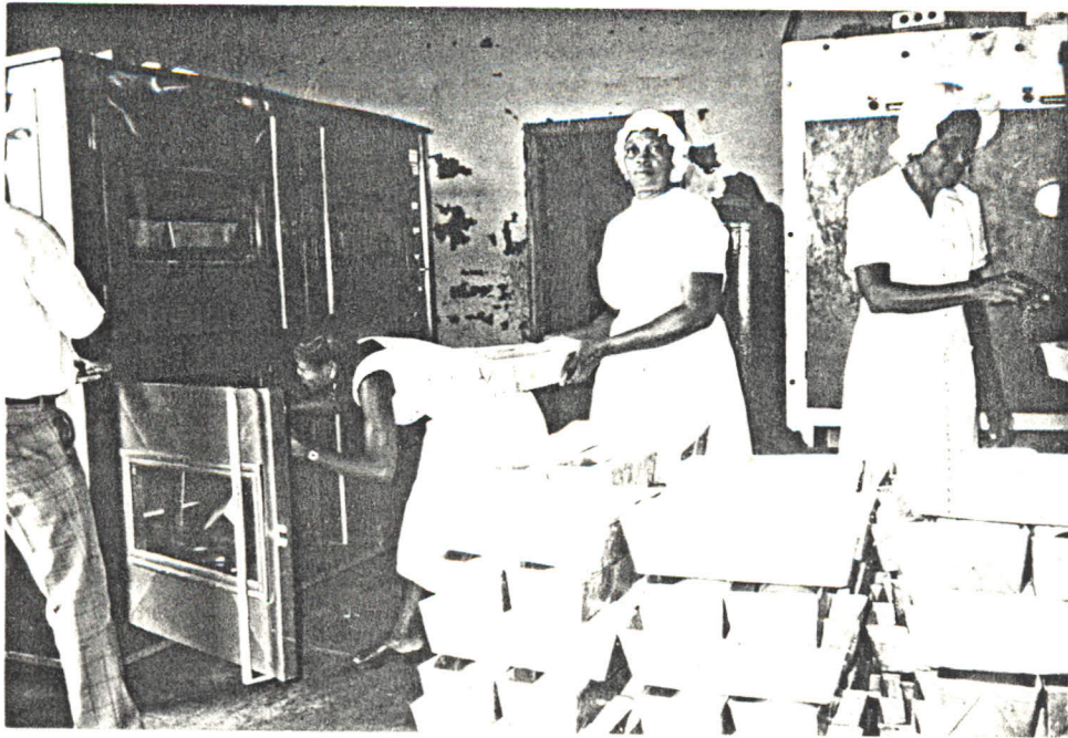
PLATE 17B: The semi-peel mode of loading being illustrated in the electric-gas oven.
