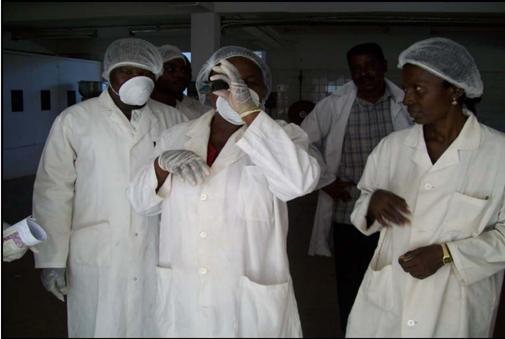
Fig 12. Trainees learning how to check soluble solids in juice with a refractometer
